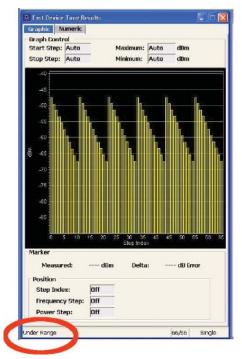
Figure 10. An under-range condition is indicated at the bottom of the graphical display.
