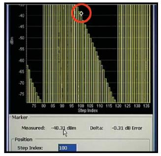
Figure 6. The Step Index setting moves the marker from one power step to the next across the range.
