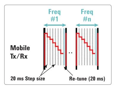
Figure 1. Fast Device Tune for W-CDMA phone calibration measures Tx power for each pre-defined 20 ms power step for a series of channels in a single frequency band.
