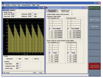
Figure 5. Application features such as a graphical display of measurement results (left) and numeric display of setup parameters (right) are part of the Fast Device Tune option.
