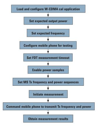
Figure 11. Example of a procedure used to make a W-CDMA Fast Device Tune measurement.
