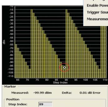
Figure 8. Enable Power Samples mode from the Fast Device Tune Setup window (upper right). The power samples are mapped to the graphical results (page 13).
