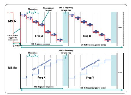
Figure 4. Example of the MS Tx and MS Rx frequency and power series for a Fast Device Tune measurement (step width = 20 ms).
